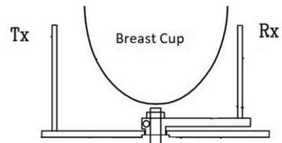
The microwave apparatus consists of a cup that holds the breast when the patient lies prone on the examination table. The transmitting (TX) and receiving (RX) antennas are located inside the hub and can be moved around the azimuth, to irradiate the breast (through TX) and capture the microwaves scattered by the breast itself (through RX). Both TX and RX are connected to a Vector Network Analyzer (VNA). No matching liquid is required
