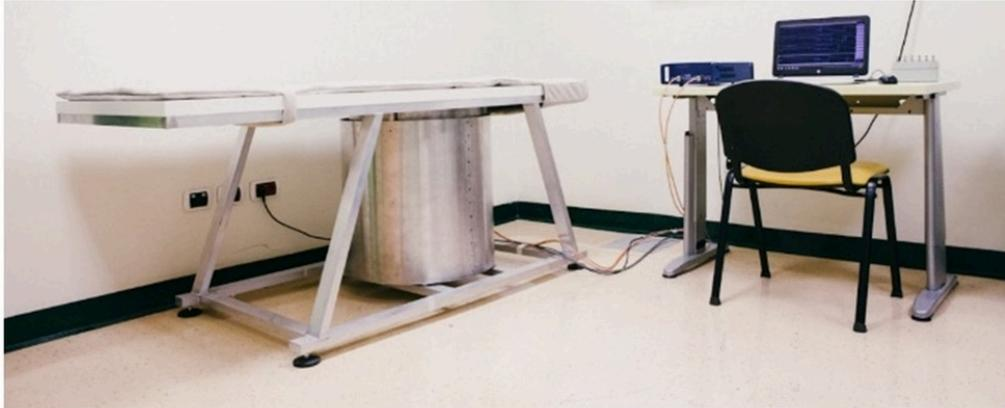
The microwave apparatus and the Vector Network Analyzer (VNA)
