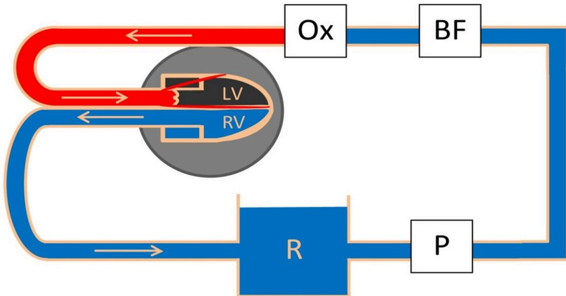
**Fig. 1:** Figure 1 Schematic representation of the Langendorff perfusion model. Blood flows from the pump (P) to the blood filter (BF) after which it is oxygenated and heated using an Oxygenator (Ox). Pressure is put on the aortic valve, and all blood traverses into the myocardium through the coronaries. Blood leaves the heart from the right ventricle and is collected in a large venous reservoir (R).
